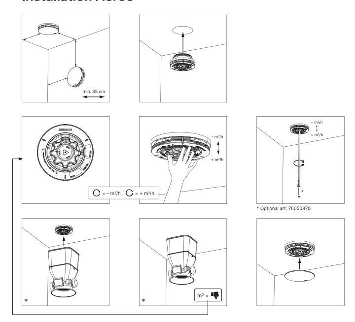
\* Correct adjustment of the ventilation air flow rates to conform with the regulations must be done with professional equipment.
